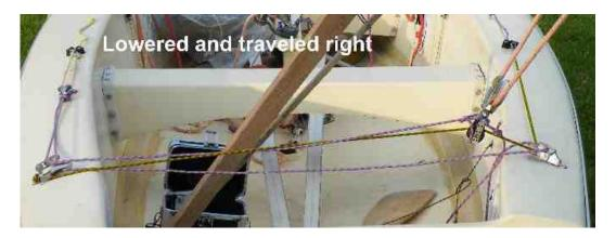
The setting of *both* the traveler height and travel distance of the traveler block will be the same on both tacks. That gives a constant "reference point" on both tacks.
