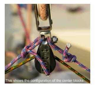
The starboard control line (yellow) controls the height of the traveler block. The port control lines (purple) limit the amount of travel (side to side).
