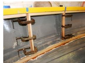
Tack on a temporary 4mm strip of plywood. This is so the thwarts can be fitted for installation after the air tanks are in.
