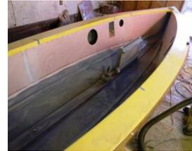
Make a small fillet with quartz micro spheres or micro balloons along the seam between the tank sides and bottom.
