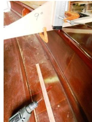
Grinding the paint off for the bottom strips.
