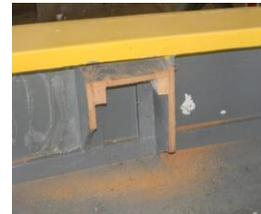
The hull with the thwarts cut and ready for the air tanks.
