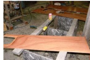
Getting ready to glue in the tank walls. Thicken the epoxy with silica thickener. You want it to fill gaps. This also shows the rear bulkhead forward of the transom.
