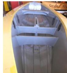
When storing your boat unscrew the dick plates so the air tanks will ventilate in case any moisture had gotten in to do any damage.
