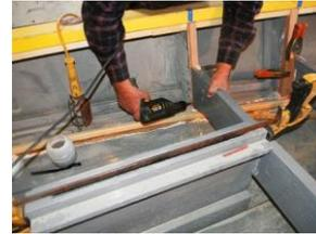
Make templates out of cheap material such as door skins. I make the tanks with three panels so the seams are mostly hidden by the front & rear thwarts.
