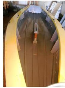
Using a laser to locate the bottom strip. The laser is set at 9 deg. to allow for any error so they won't go beyond the 10 deg. limit. Drill small pilot holes on 6" centers for the screws. Drill them 1/2" to the outside of the laser mark.
