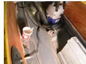
Thwarts are back in, access plates are installed and tanks are painted. A good source for deck plates is Beckson Marine, go to their over-run section for the deals.
