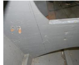
Cutting with a portable jig saw. I finished the cuts where the saw wouldn't reach with a Japanese pull saw.
